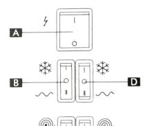
A. Main switch: it is used to switch on/off the power supply to the whole machine A.
